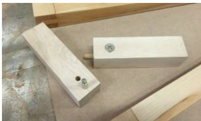
Figure 51: Testing of MINIFIX 15 Connectors
