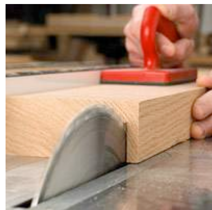
Figure 3: Table Saw - Rip Cut (Wood Magazine, 2010)
