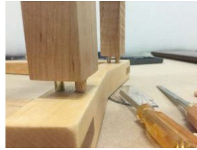
Figure 52: Assembling of MINIFIX 15 Connectors
